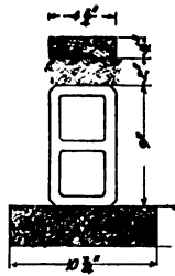
Fig. 57.—McRoy Tile, 2-Duct Conduit, Class "B" Construction.
