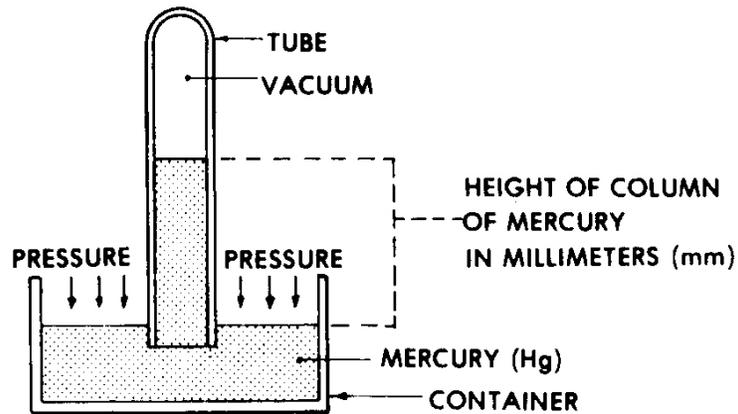
Figure 5-1. "Millimeters of mercury" as a measure of pressure.
