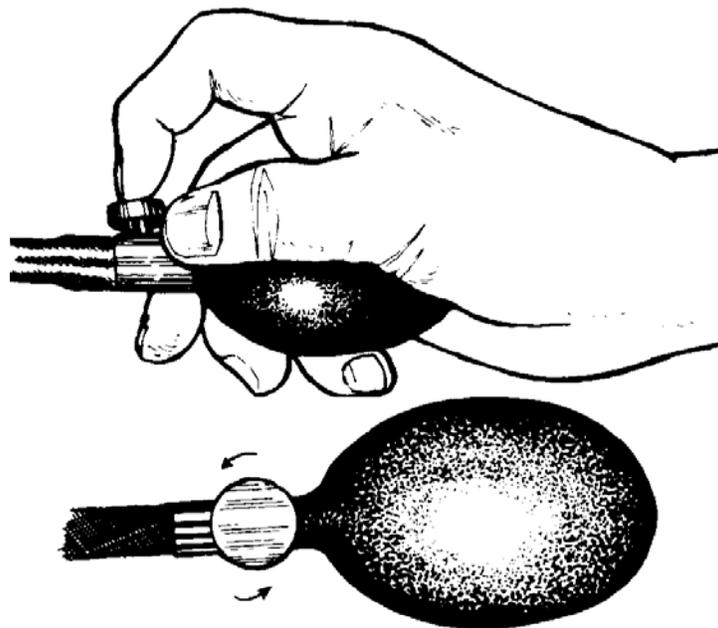
Figure 5-10. Rotating the screw counterclockwise to release pressure.
