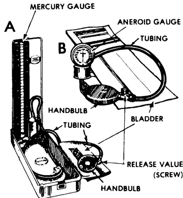
A Portable mercury sphygmomanometer.
