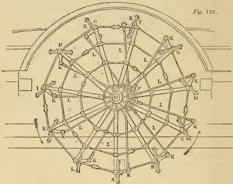
between each radial arm L and the short paddle-arm K is capable of being changed by any motion imparted to L: the radial arms are connected at the other end with a centre, round which they are capable of revolving.
