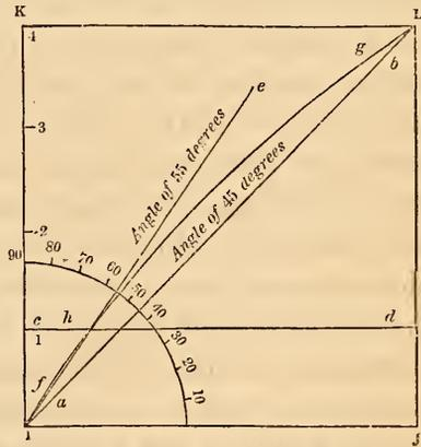
From the angle I of the square draw the line I, *e* at an angle of fifty-five degrees with the line I, J, and where the line I, *e* intersects the horizontal line *c, d*, at the point *h*, it gives a point through
