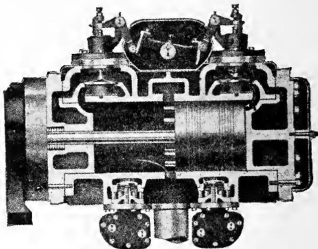
Fig. 35. Cylinder and Valve Arrangement in Skinner Uniflow Engine.
