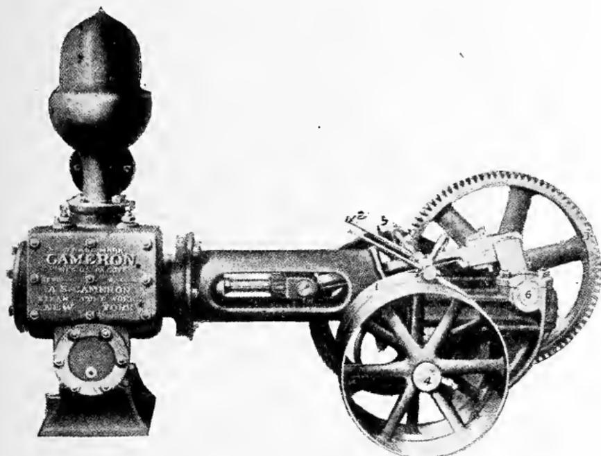
Fig. 49 Belt-Driven Power Pump
