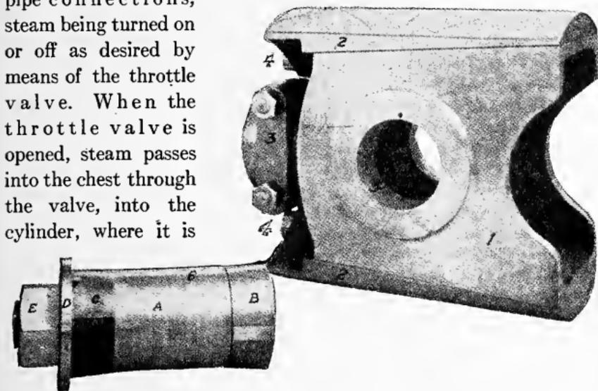
Fig. 14. Typical Crosshead and Pin for Large Size Engine
