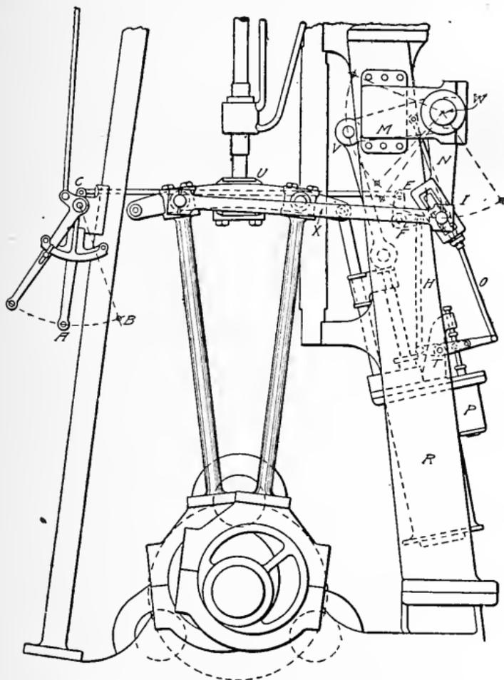
Fig. 64. Details of Steam Starting Gear
