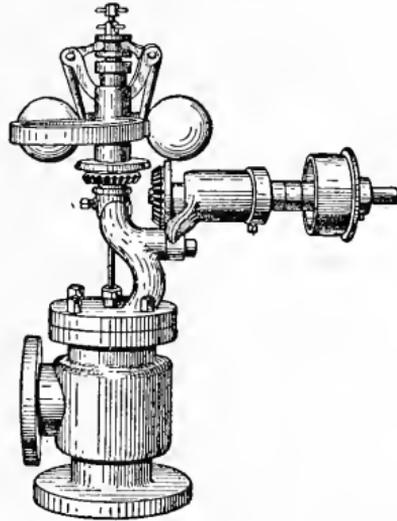
Fig. 91. Waters Spring Type of Fly-Ball Governor
