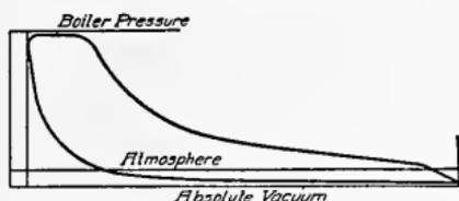
Fig. 32. Indicator Card for Uniflow Engine Operating Non-Condensing
