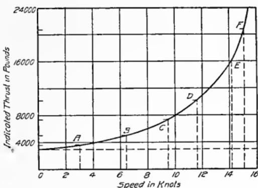
Fig. 66. Curve Showing Indicated Thrusts for Different Speeds
