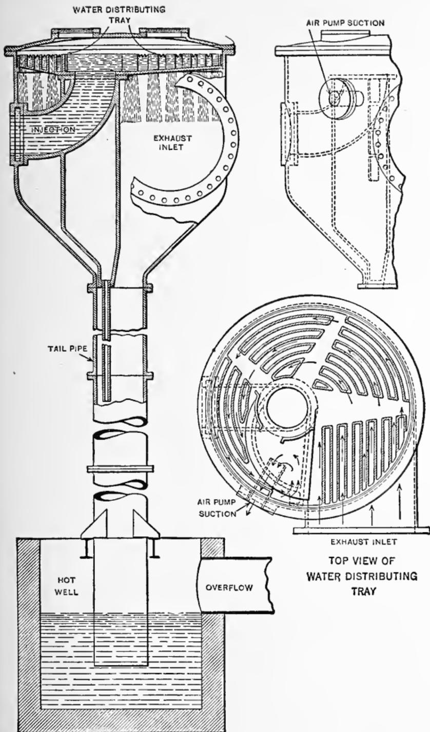
Fig. 80. Alberger Barometric Jet Condenser
