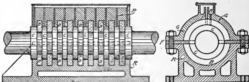
Fig. 62. Typical Marine Thrust Bearing
