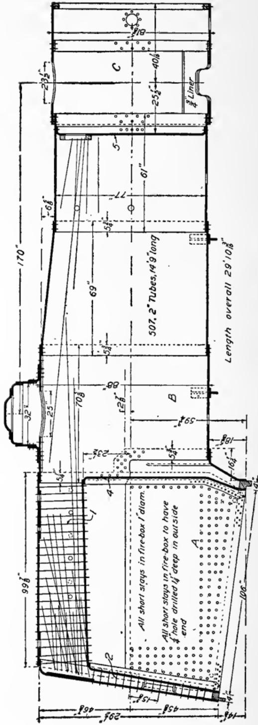
Fig. 47. Detailed Drawing of Modern Locomotive Boiler
