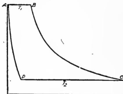
Fig. 70. Theoretical Indicator Diagram
