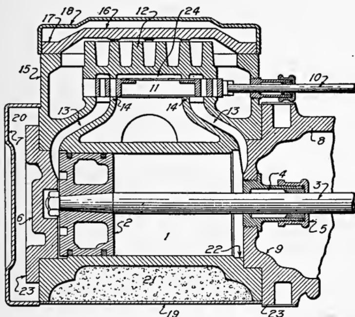
Fig. 8. Cylinder and Valve Mechanism Shown in Section
