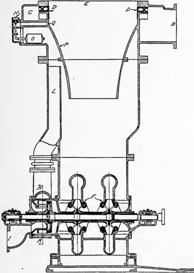
Fig. 81. Cross Section of Leblanc Jet Condenser
