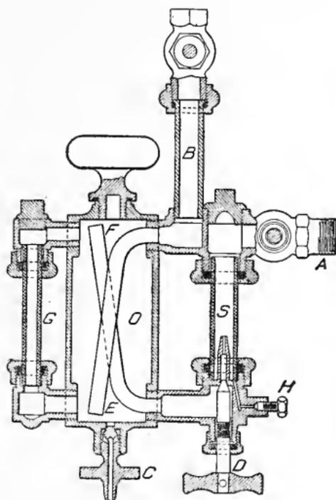
Fig. 99. Section of Sight-Feed Lubricator
