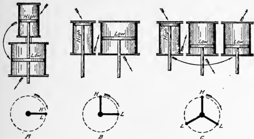
Fig. 54. Diagrams of Tandem and Cross-Compound Cylinder Arrangements
