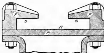
Fig. 60. Type of Marine Crosshead Guide
