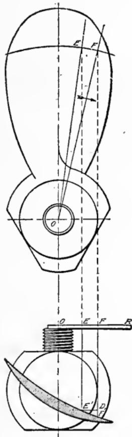
Fig. 68. Typical Shape of Propeller Blade
