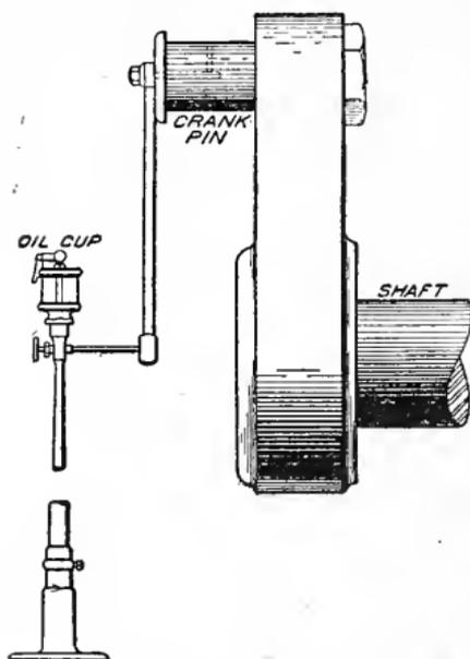
Fig. 98. Centrifugal Oiler
