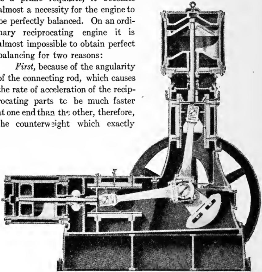
Fig. 29. Section of Angle-Compound Engine
