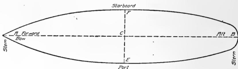
Fig. 53. Plan of Vessel Showing Different Parts
