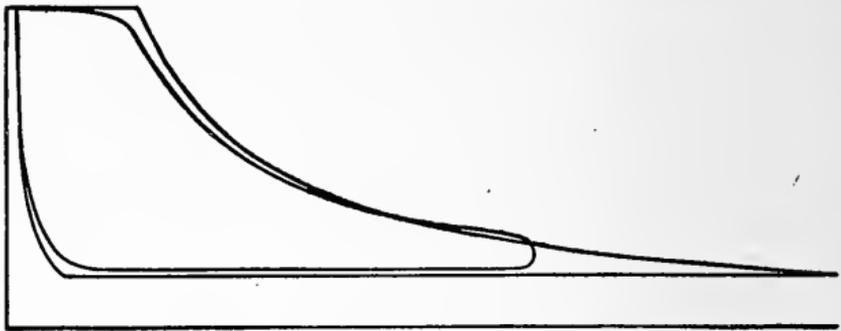
Fig. 71. Superposed Ideal and Actual Indicator Diagrams
