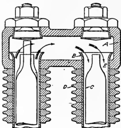
Fig. 74. Section of Foster Superheater Tubes
