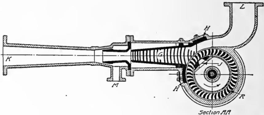
Fig. 82. Section of Leblanc Condenser Taken through *AA*, Fig. 81
