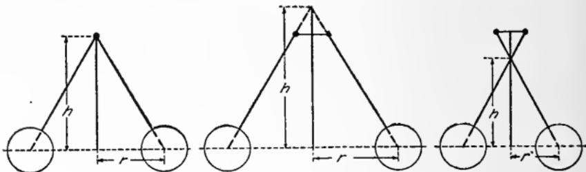
Fig. 86. Diagrams Showing Action of Pendulum Governor
