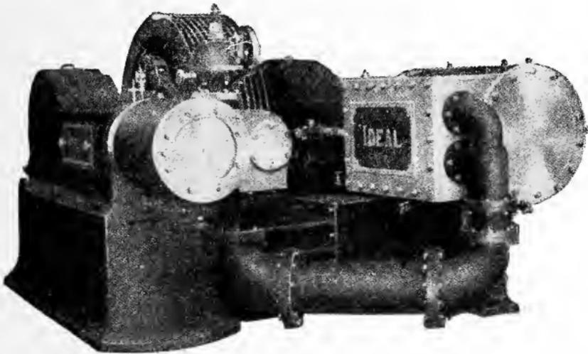
Fig. 20. Typical Cross-Compound Engine
