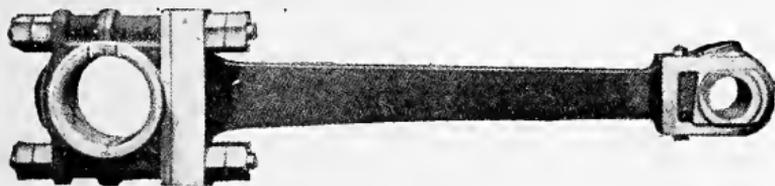
Fig. 16. Marine Type of Connecting Rod
