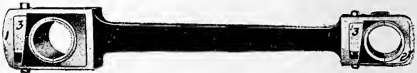
Fig. 15. Solid Forged Steel Connecting Rod
