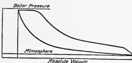
Fig. 31. Indicator card for Uniflow Engine Operating Condensing
