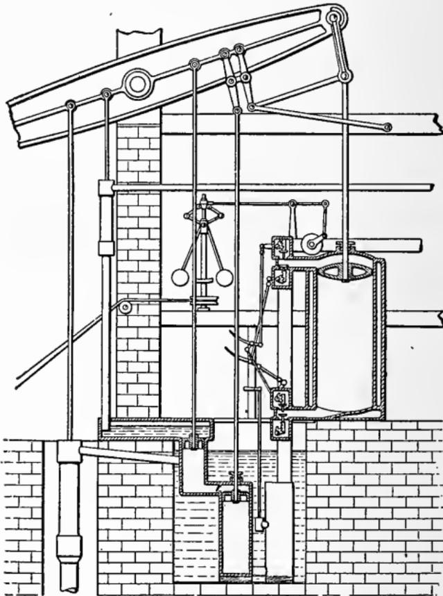
Fig. 4. Final Form of Watt's Steam Pumping Engine
