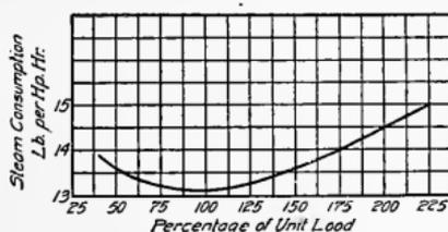
Fig. 34. Economy Curve for Uniflow Engine Operating Non-Condensing
