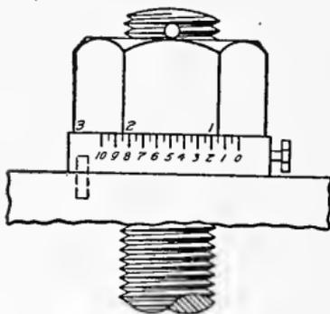
Fig. 69. Marking Nuts and Washers
