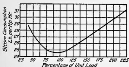
Fig. 33. Economy Curve for Uniflow Engine Operating Condensing
