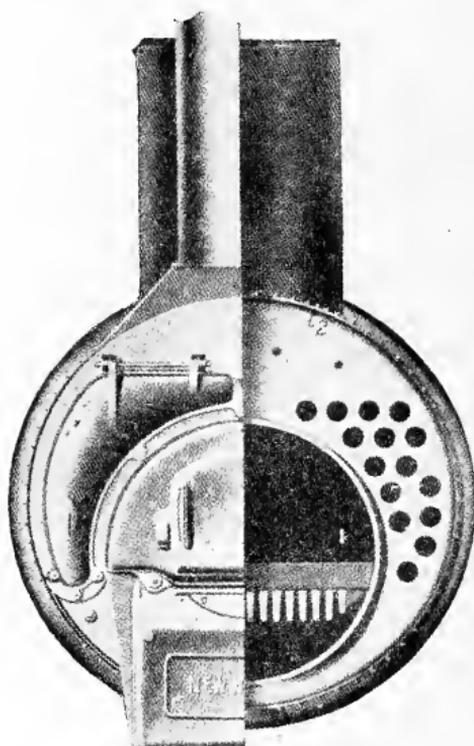
Fig. 44. End View of Modified Scotch Marine Boiler
