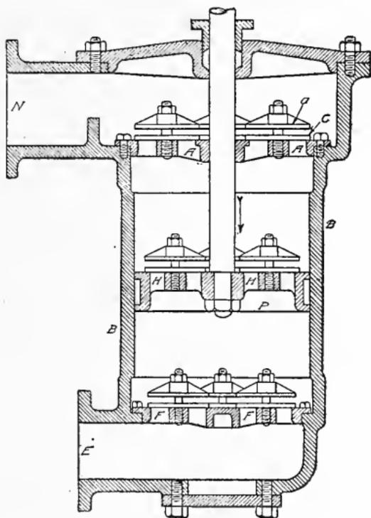
Fig. 65. Section of Air or Vacuum Pump
