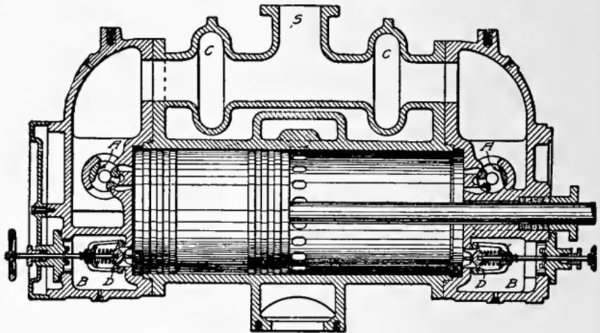
Fig. 30 Sectional View of Uniflow Engine
