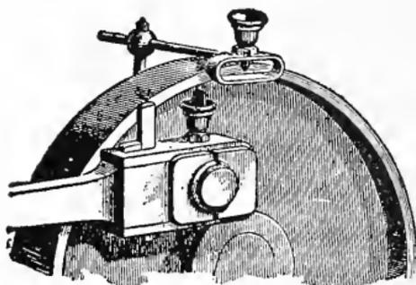
Fig. 97. Form of Wiper Crank Pin Oiler
