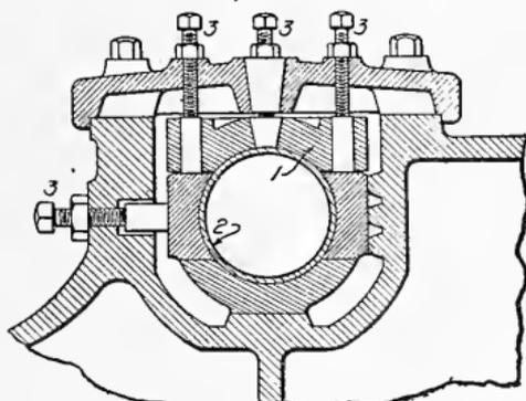
Fig. 18. Section of Babbitt Lined, Quarter-Boxed Main Bearing
