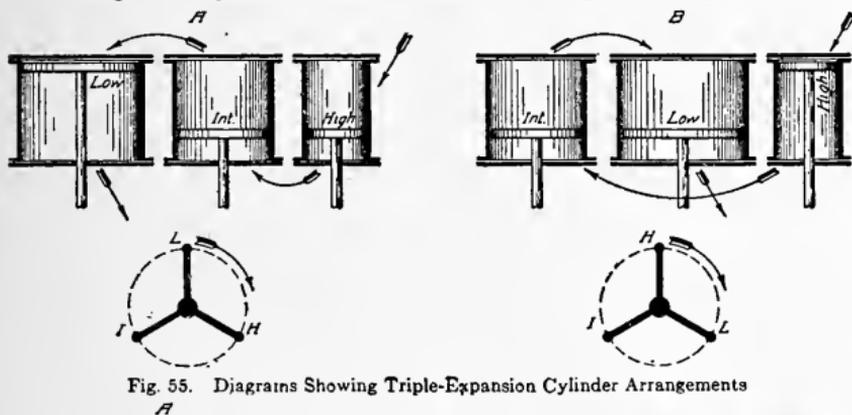
Fig. 55. Diagrams Showing Triple-Expansion Cylinder Arrangements
