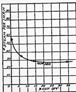
Fig. 108. Steam Consumption for Different Cut-Offs
