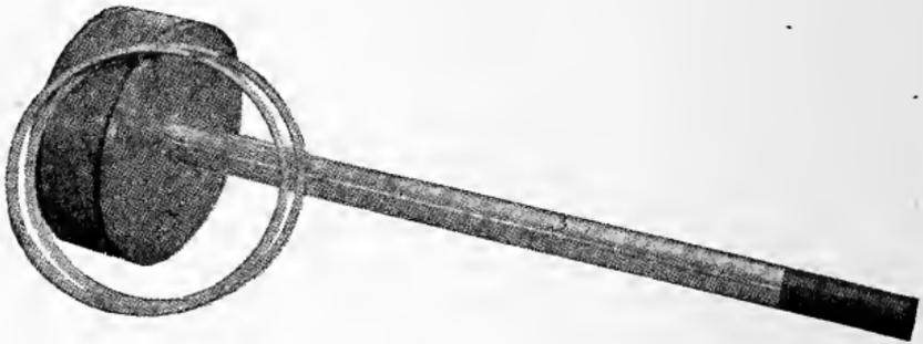
Fig. 9. Piston, Showing Piston Rings for Making Steam-Tight Joints
