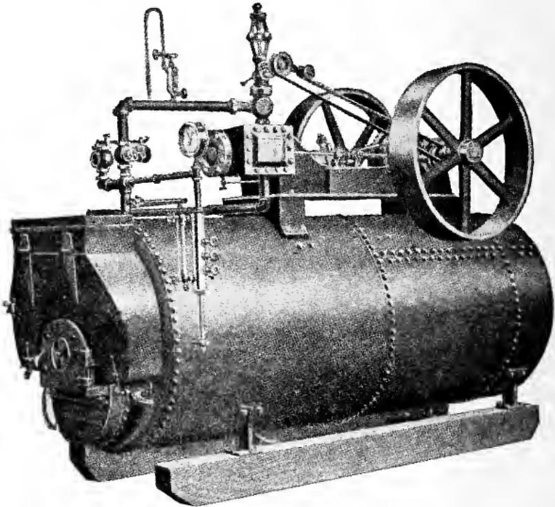
Fig. 46. Semi-Portable Engine and Boiler
