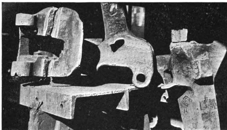
FIG. 23.—Car coupler used in railway work before arc welding.
