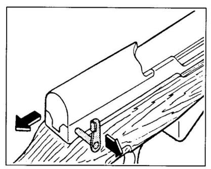
2 To field strip, clear the chamber and unload magazine. Depress follower (31) and ease bolt closed. Swing takedown latch (14) up and pull out. Ease rear housing (17) off. Pull out recoil spring assembly (24-27). Pull bolt carrier (18) and bolt (19) to rear and remove.
