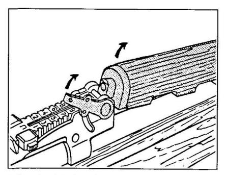
4 Insert point of cartridge into hole of the handguard catch (7) and rotate catch up as shown in illustration. Lift up rear of handguard (2), and pull it free of barrel. Then push piston (1) out of gas cylinder. Pivot bayonet (9) to middle position, and remove cleaning rod (55).
