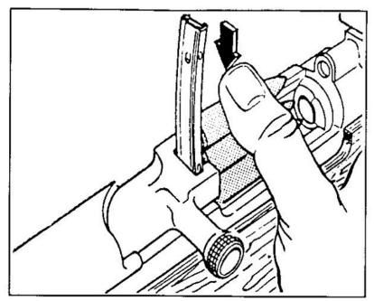
1 The SKS has a fixed box magazine (30). To load, open action by pulling back bolt carrier (18). Insert a loaded stripper clip into clip guides of bolt carrier and push cartridges down into magazine as shown. The magazine can also be loaded with loose cartridges.
