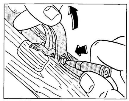
3 For further disassembly, cock hammer and put carbine on safe. Turn carbine upside-down and push in on trigger guard latch (15) with cartridge nose or punch. When latch is pushed in sufficiently, the trigger guard (39) should jump out slightly. Guard can then be pulled free.
