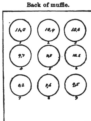
FIG. 3.—Position of cupels in muffle.
