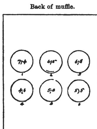
FIG. 4.—Position of cupels in muffle.
