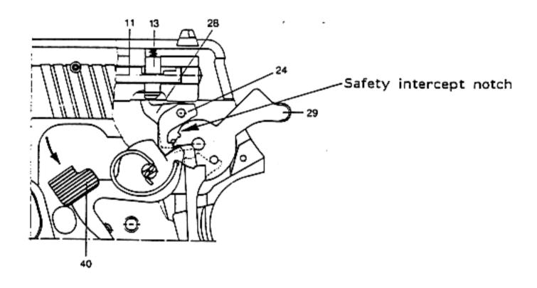
Function of the decocking lever and safety notch
