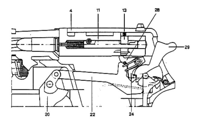
Function of the firing pin lock
