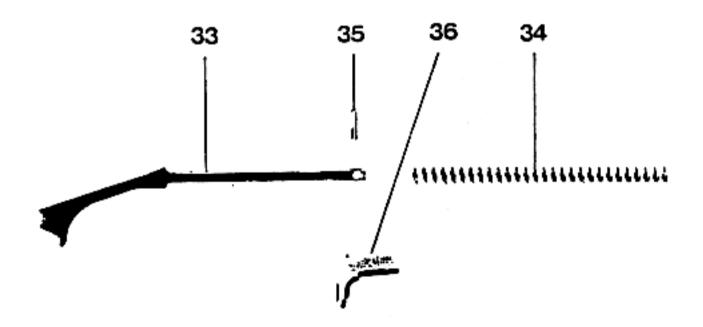
Hammer strut with main spring and main spring seat
