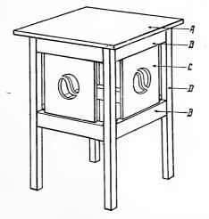
FIG. 124.—PARTS OF A PIECE OF FURNITURE. A, TOP; B, RAIL; C, PANEL; D, LEG OF SUPPORT.
