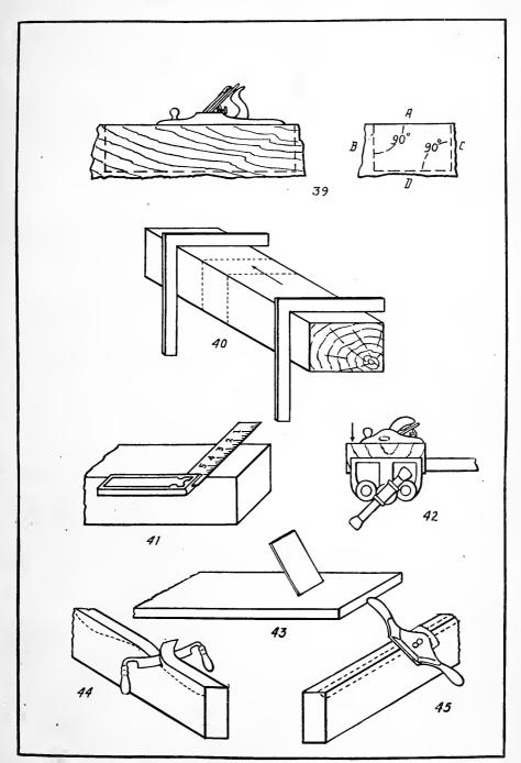
FIG. 39.—SQUARING STOCK. FIG. 40.—TESTING WITH SQUARE. FIG. 41.—MARKING END, FIG. 43.—USE OF CABINET SCRAPER. FIG. 44.—USE OF DRAW KNIFE. FIG. 45.—USE OF SPOKE SHAVE, Wood Chisel.—No tool has yet been devised to replace the wood chisel, and for years to come it will be used universally for gaining, mortising, beveling and for re-
