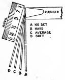
FIG. 200.—SAW SET Showing Degree of Set. types. In the Morrill saw sets the principal of compression is employed, making the steel stronger and more homogenous. (See Fig. 199.)
