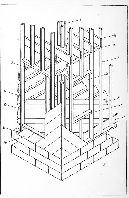
FIG. 150.—FRAME OF HOUSE (WITH T-SILL).
