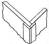
FIG. 116.—BUTT JOINT (CLEATED).
