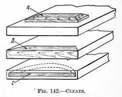
edge all the way around the piece. These strips are put on by the use of glue and screws. C, in Fig. 142, shows the common method used in cleating thin doors, sliding leaves, etc. They are usually made by feeding the end of the door into a circle saw and then cutting a spline to match.
