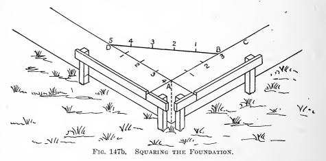
location by driving a stake. To this stake attach a line and run it past the next corner of the building and parallel with the street. Run a line back from the street from the first corner, A, in Fig. 147a, at right
