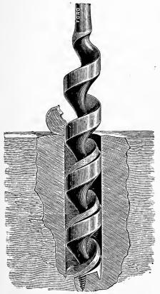
FIG. 214.—CUTTING ACTION OF A BIT.
