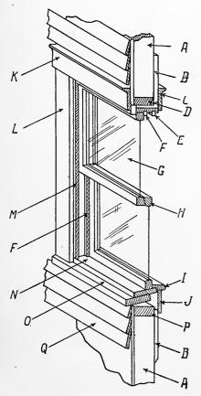
FIG. 153.—CROSS SECTION OF A WINDOW FRAME.
