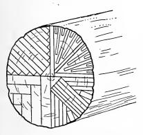
FIG. 243.—METHODS OF QUARTER-SAWING LUMBER.
