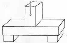
FIG. 123 .--- DIRECTION OF TRANSVERSE STRESS.
