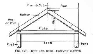
*Pitch.*—The angle of incline of the common rafter is called the pitch of the roof. The most common rafter pitches are given in the following table by the rise and run of the common rafter.
