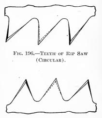
FIG. 197.—TEETH OF CUT-OFF SAW (CIRCULAR).
