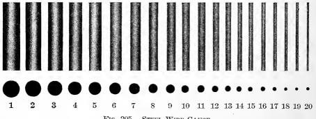
FIG. 205.—STEEL WIRE GAUGE.
