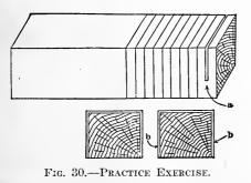
and steadying the blade of the saw with the first finger of the left hand. This will make a slight kerf, which can be increased with a light pushing stroke. At each succeeding stroke, gradually lower the handle end of the saw until a horizontal position is gained. The sawing in all cases must be done with a light lifting stroke, without any forcing into the wood, using long steady
