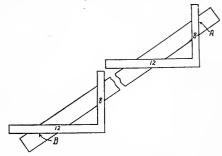
FIG. 181.—SIDE CUTS OF RAFTERS. A—Square set for side cut. B—Square set for plumb cut. Valley Rafter.—The valley rafter, E in Fig. 179, is the hypothenuse of the right-angled triangle formed by the common rafter with the ridge, corresponding with the right-angled triangle formed by the hip rafter, common rafter and plate; therefore, the rules for the lengths and cuts for valley rafters are the same as for hip rafters. The side cuts are also the same as for hip rafters.
