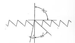
FIG. 191.—RIP-SAW TEETH, SHOWING ONE-HALF PITCH.
