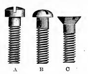
FIG. 206.—MACHINE SCREWS. a—Flat Head; b—Oval Plumber's Head; c—Fillister Head.
