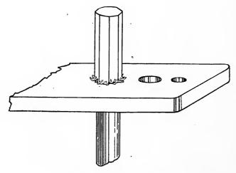
FIG. 99.—USE OF, A DOWEL PLATE.
