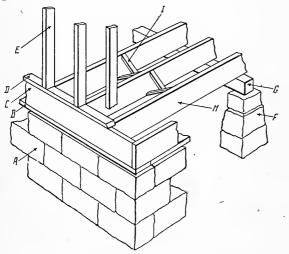
FIG. 149.—FOUNDATION FRAME. (Box SILL.) A.—Foundation D.—lower plate G.—beam B.—foundation plate E.—stud H.—joist C.—sill F.—pier I.—bridging
