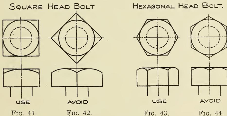
usually drawn. The views of Figs. 41 and 43 are usually preferred because they indicate more clearly in the elevation that the heads are square or hexagonal. Figs. 42 and 44 both have two faces showing in the elevation and therefore might be confused.
