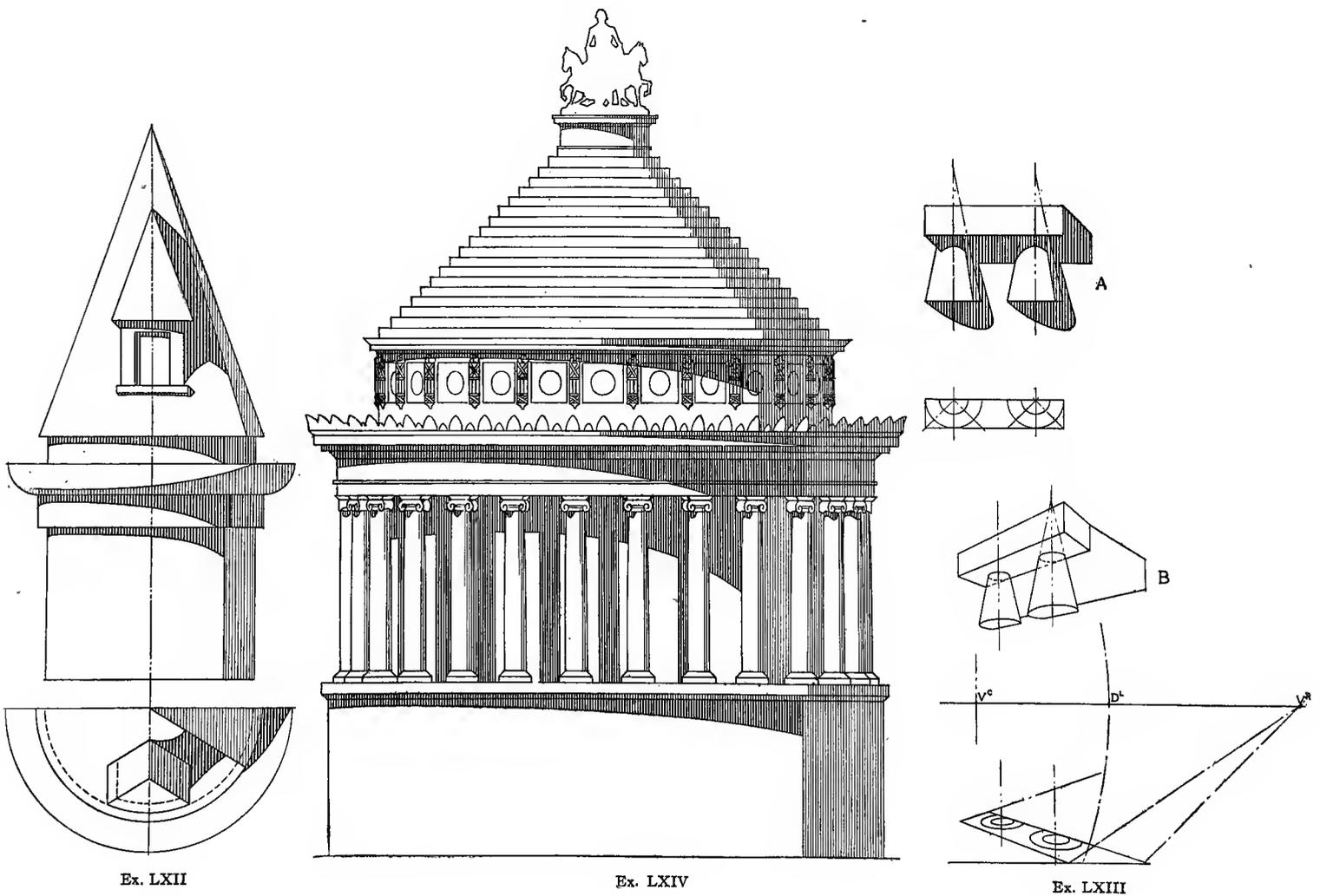
Hollow Cones play even a less conspicuous part in Architecture than do Solid Cones, neither the larger features nor the details of ornamentation often assuming this form. The only noticeable cases are the Conical Niche, the Conical Pendentive, and Curved Pediments.
