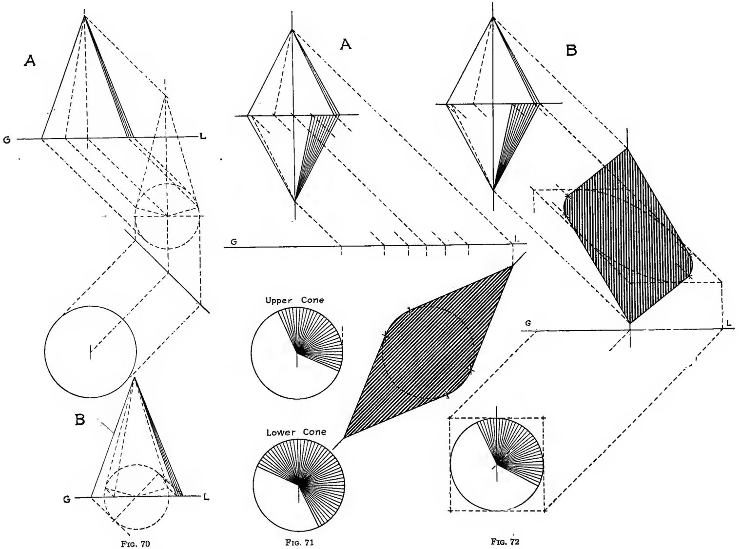
98. Fig. 70 A and B shows how the same result is obtained by M. Pillet by means of the auxiliary 45-degree Plane of Projection, described in Chapters III and IV, and illustrated in Figs. 24 and 47.
