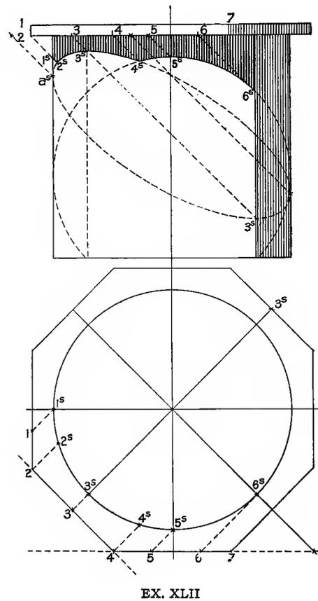
*Example XLIII. A Semicircular Shelf Upon a Semi-octagonal Pillar. Plan and Elevation.*
