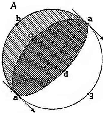
The Hollow Hemisphere, on the other hand, has upon its concave surface three lines, all of which are Great Semi-Circles, namely, (1) the Line of Shade upon the rim, which casts the shadow; (2) the Line of Shade and Shadow, which divides the shade from the shadow; and (3) the Line of Shadow, which divides the shadow from the light.
