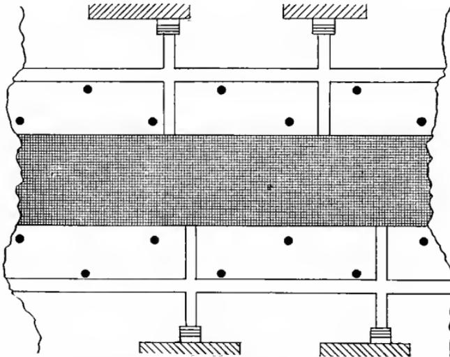
FIG. 13. — Plan of modern avenue provided with a 40-foot roadbed, 6-foot sidewalks, 23-foot tree belts, with alternating rows of trees 60 feet apart.
