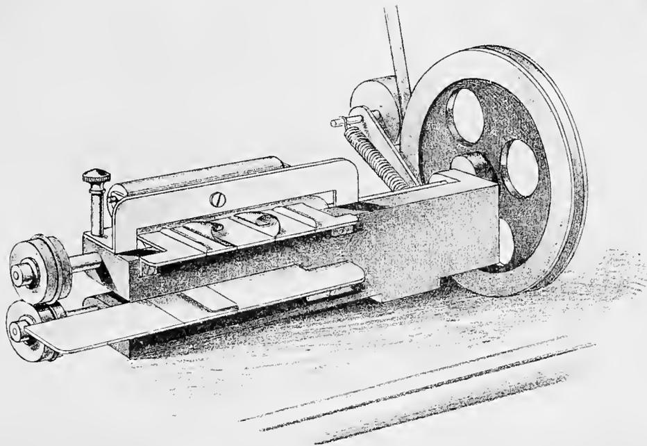
THE ROTARY CUTTER AND SELF FOLDING ATTACHMENT,
