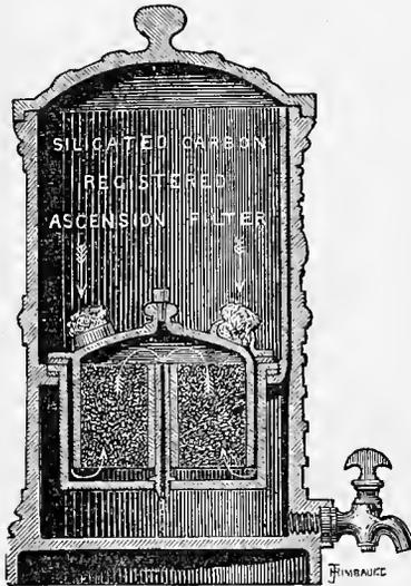
carbon in the directions shown by the arrows in the illustrations. When cleansing the filters, the small india rubber peg should be removed and placed in the socket at the bottom; the carbon should be strongly blown in from the top, and scrubbed with a brush and boiling water. All the parts are kept in stock by the company, and therefore new carbon media can be supplied without the filters being returned to the makers.
