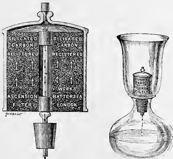
can be taken out, when, with the aid of a piece of indiarubber tube, they can be converted into pocket filters, the small indiarubber peg at the top being placed in the socket-hole at the bottom. The water passes through the carbon in the directions shown by the arrows in the illustrations. When cleansing the filters, the small indiarubber peg should be removed and placed in the socket at the bottom; the carbon should be
