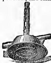
Showing **PLUNGER**, which works up and down in tub about 60 times per minute, atmospherically forcing the hot water and soap through the clothes, thus not only loosening the dirt but thoroughly removing it in a short space of time, without any possibility of wearing or injuring the most delicate articles.
