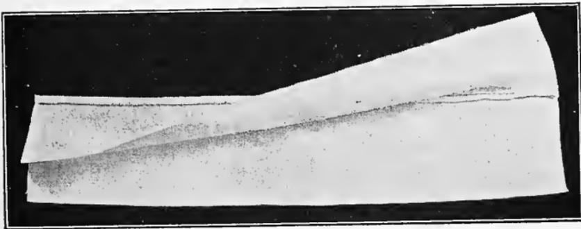
MACHINE-MADE FRENCH SEAM
