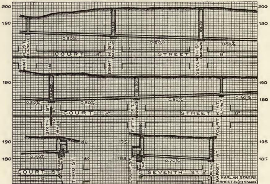
Fig. 39. Typical Sewer Profile Sheet.
