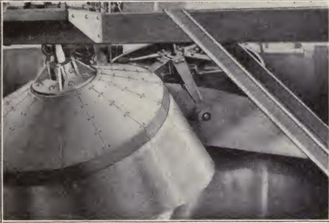
Fig. 44. Reinsch-Wurl Screen in Experimental Plant, Dresden, Germany
