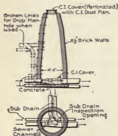
Fig. 9. Sectional Elevation and Plan of Sewer Manhole.
