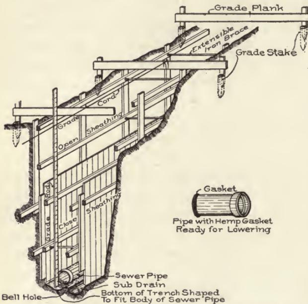
Fig. 40. Diagram Showing Construction of Pipe Sewer.
