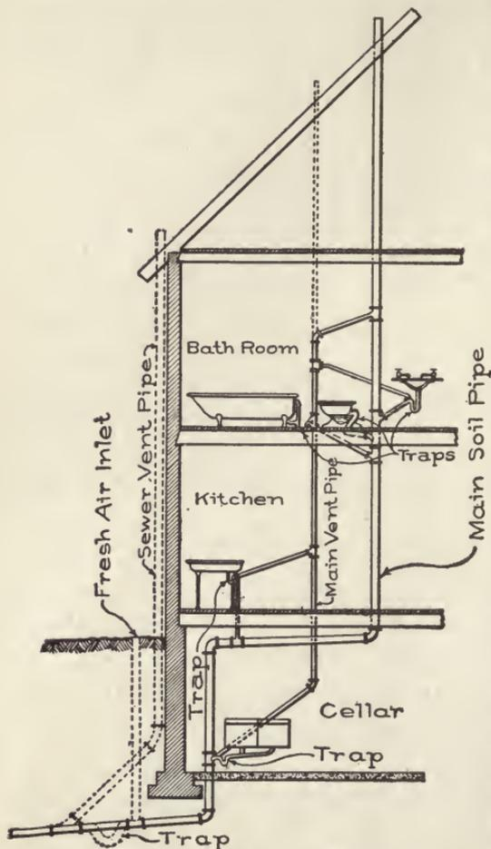
Fig. 35. Diagram of House Sewerage System.
