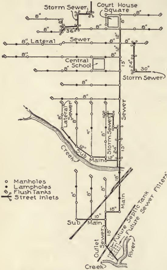
Fig. 4. Kinds of Sewers and Arrangement of Accessories.
