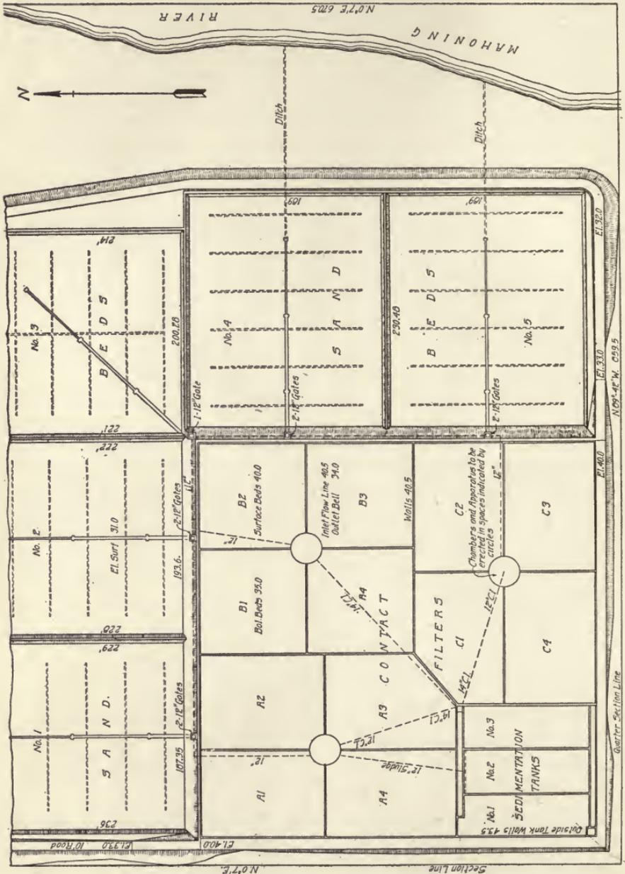
Fig. 66. Plan of Sand Filters at Alliance, Ohio
