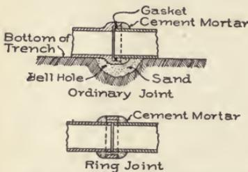
Fig. 17. Joints in Pipe Sewers.
