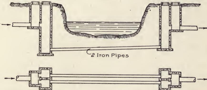
Fig. 15. Sectional Elevation and Plan of Inverted Siphon.
