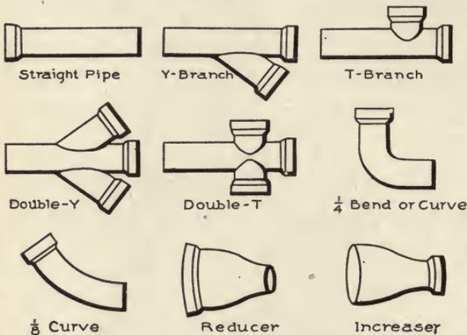
Fig. 16. Vitrified Sewer-Pipe and Specials.
