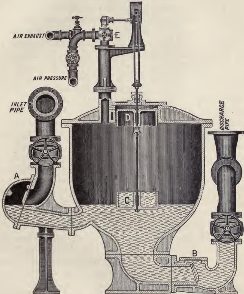
Fig. 73. Detailed Section of Shone Automatic Ejectors
