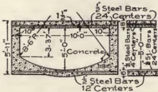
Fig. 22. Ingersoll Run Sewer with Low Headroom, Des Moines, Iowa.
