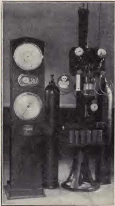
Fig. 70. Automatic Control Apparatus for Liquid Chlorine
