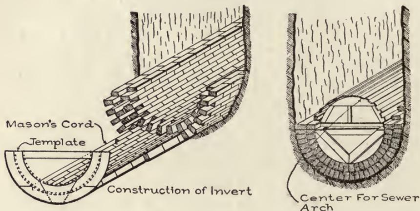
Fig. 41. Diagrams Showing Construction of Brick Sewer.
