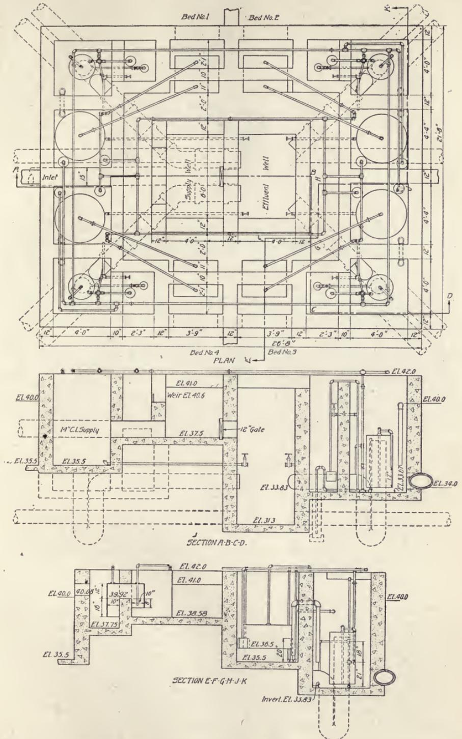
Fig. 58. Plan and Sections of Automatic Control Chamber for Contact Beds at Alliance, Ohio
