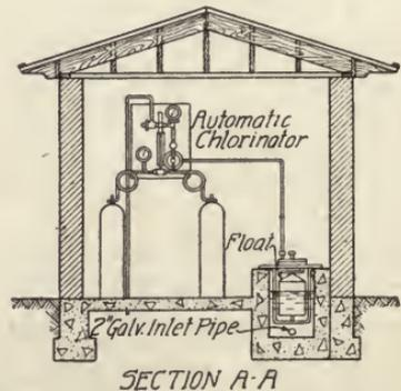
Fig. 69. Plant and Sections of Disinfection Plant
