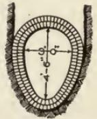
Fig. 19. Egg-Shaped Brick Combined Sewer.
