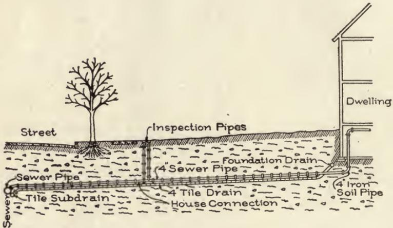
Fig. 6. Street Sewer, Subdrain, and House Connection.
