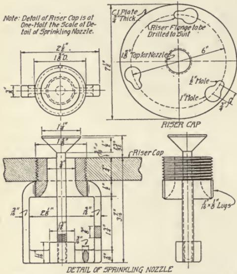
Fig. 65. Details of Sprinkling Filter Nozzle
