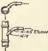
Fig. 7. Junction of House Connection with Sewer.
