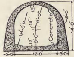
Fig. 23. Dry-Run Sewer, Waterloo, Iowa.
