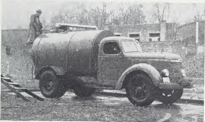
Figure 5.—Sewage sludge containing 6 to 10 percent of solids is transported to farms from the Richmond, Ind., disposal plant.
