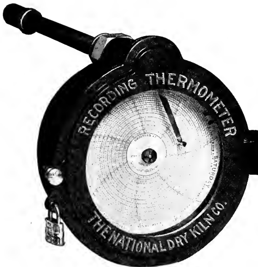
Fig. 97. The Recording Thermometer.
