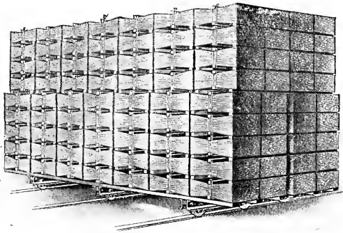
Fig. 59. Method of loading Kiln Car with Shingles cross-wise of Dry Kiln.
