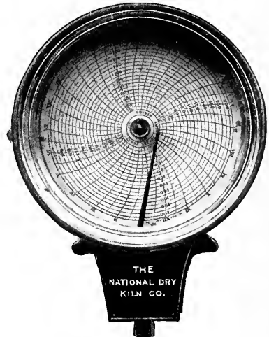
Fig. 99. The Recording Steam-Pressure Gauge.
