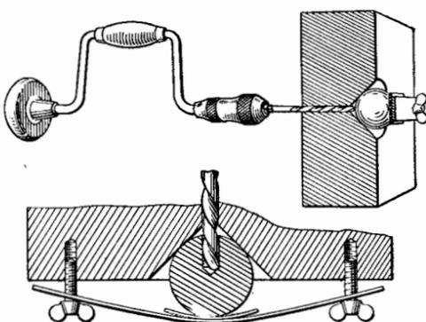
A METHOD OF DRILLING HOLES IN MARBLES.
