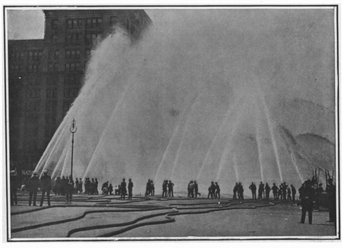
Twenty-four Streams with a Capacity of Over 18,000 Gallons per Minute.
