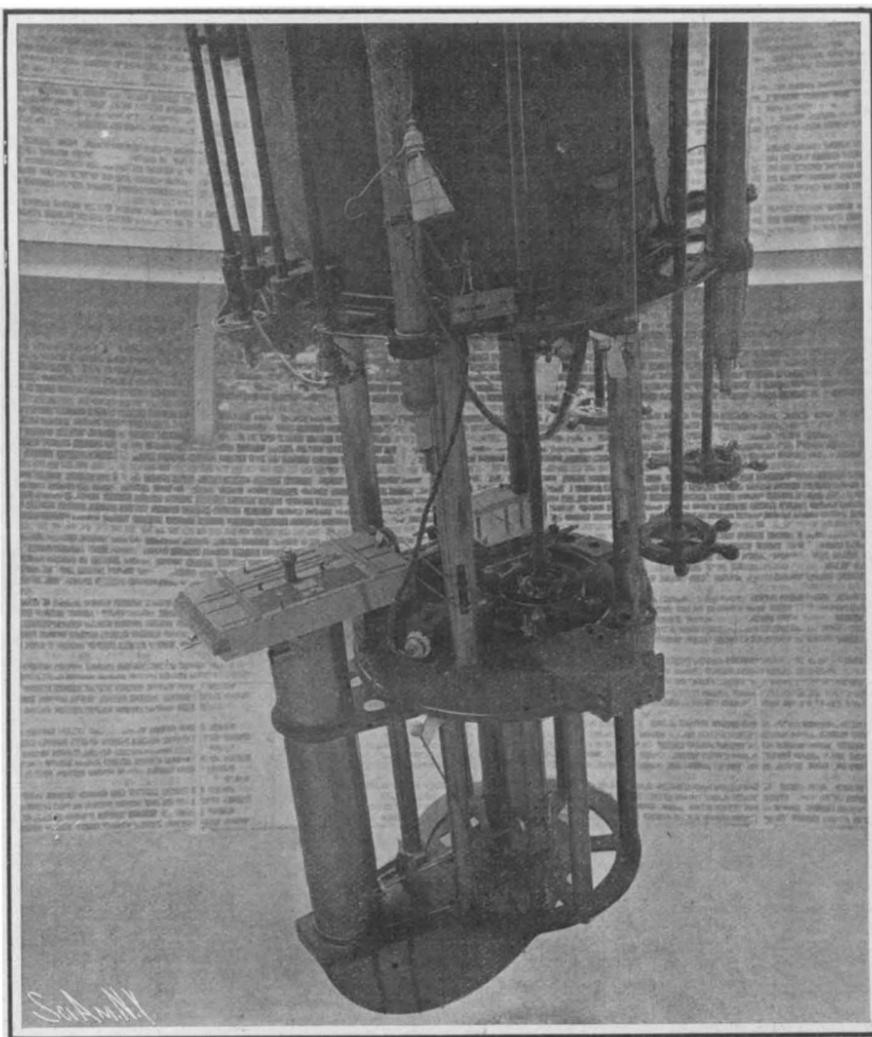
In principle the instrument is a spectroscope, but with the addition of a second slit placed close in front of the photographic plate. The second slit cuts off all but that portion of the solar spectrum to be photographed.
