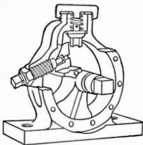
Fig. 7.—Hotchkin Shock Absorber With Cover Removed and Section Broken Away to Show Check-valve and By-Pass.
