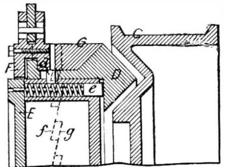
Friction Band in Position for Low Speed.
