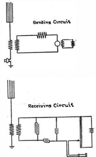
**Fig. 2.—Connections for Direct System.**
