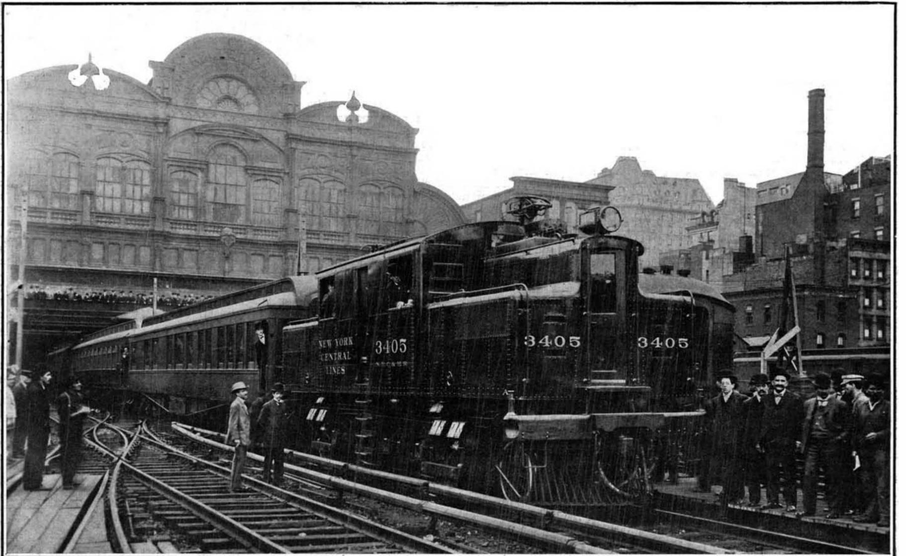
The locomotive, of 3,200 maximum horse-power, weighs 95 tons and can exert twice the horse-power of the express steam locomotives of the road.
