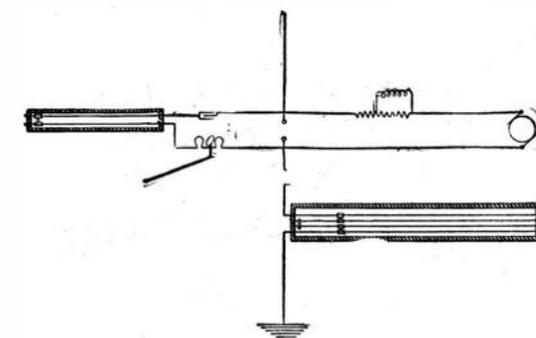
**Fig. 1.—Diagram of Arc Method of Transmission.**
