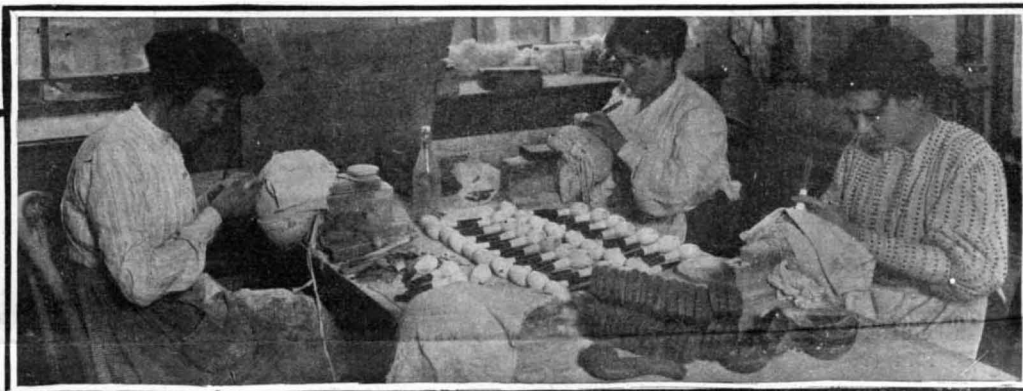
Smoothing Off the Pipes with Shave-Grass.
