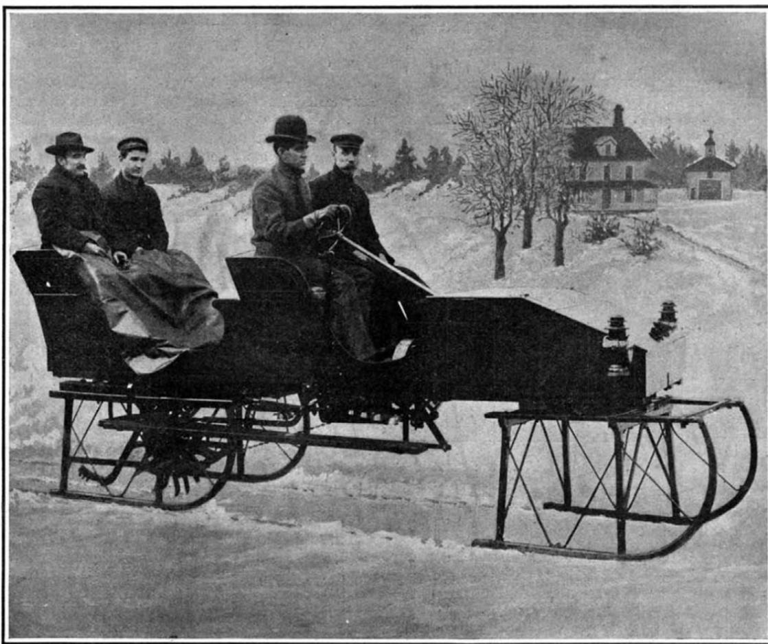
MOTOR SLEIGH SAID TO BE CAPABLE OF MAKING 35 MILES AN HOUR ON SNOW AND 90 MILES AN HOUR ON ICE.
