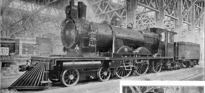
Cylinders, 143° and 33% inches by 253° inch stroke. Diameter driving wheels, 805° inches. Heating surface, 2,617 square feet. Weight, 161,700 pounds.
