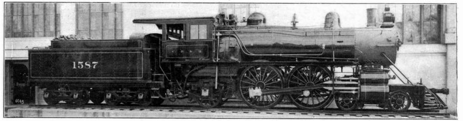
Cylinders: high-pressure, 15 inches; low-pressure, 25 inches. Stroke, 26 inches. Diameter driving wheels, 841/4 inches. Heating surface, 3002.5 square feet. Steam pressure, 210 pounds. Weight of engine, 183,080 pounds.
