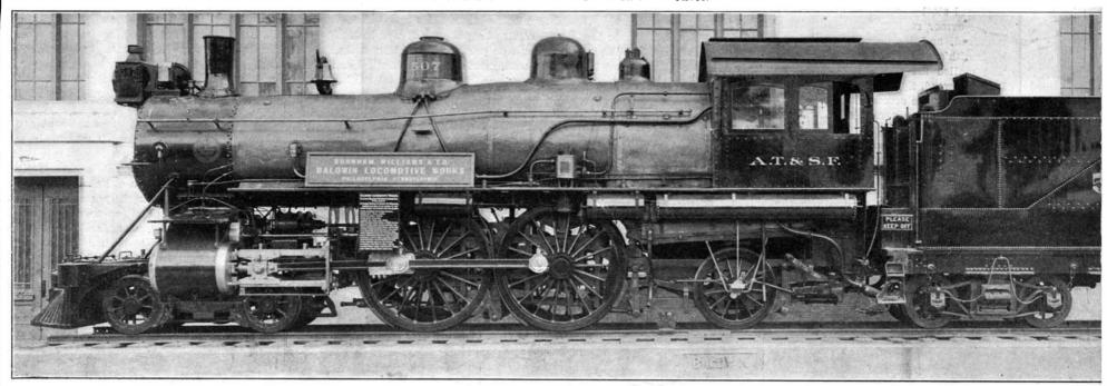
Cylinders: high-pressure, 15 inches; low-pressure, 25 inches diameter. Stroke, 26 inches. Diameter driving wheels, 79 inches. Heating surface, 3,206 square feet. Pressure, 220 pounds. Weight, 19 Four-cylinder Balanced Compound, for the Atchison, Topeka & Santa Fé Railway System.
