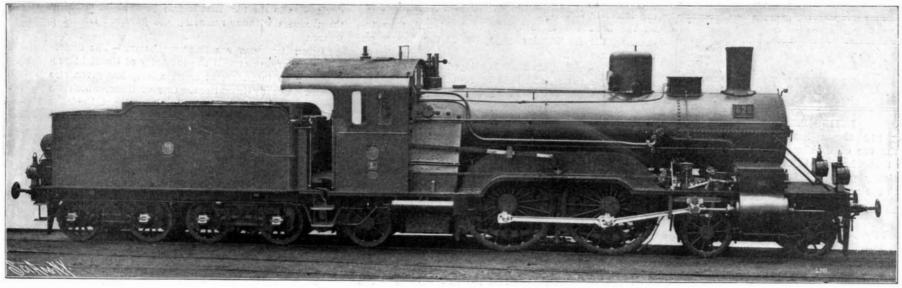
Cylinders, 14 and 24 inches by 24 inch stroke. Diameter driving wheels, 6 feet 6 inches. Heating surface, 1.922 square feet. Weight, 132,700 pounds. Four-cylinder, Balanced, Compound German Engine, with Superheater.
