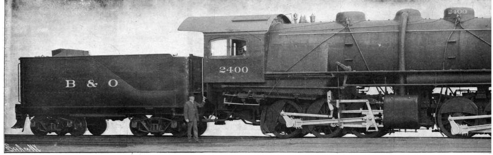
Cylinders, z0 and 52 inches diameter by 32-inch stroke. Diameter of boiler, 7 feet. Heating surface, 5,586 square feet. Working pressure, 235 pounds. Weight of engine, all available for adhesion, 334,500 pounds. B. & O. Freight Locomotive, the Heaviest and Most Powerful Locomotive Ever Built.
