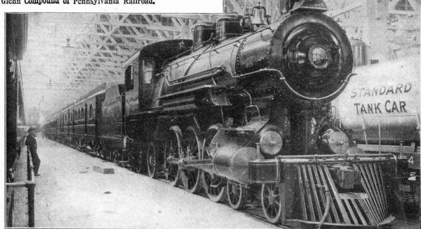
Cylinders, 20 x 26 inches. Driving wheels, 69 inches diameter. Heating surface, 2,930 square feet. Working pressure, 200 pounds, Weight of engine, 183,200 pounds.
