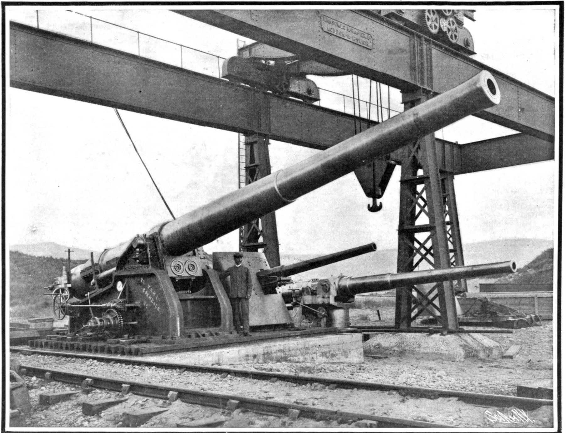
**Length Over All, 37.2 feet. Diameter at Breech, 36 inches. Diameter at Muzzle, 18 inches. Weight of Gun, 28 tons. Weight of Projectile, 380 pounds. Muzzle Velocity, 2,900 feet per second. Muzzle Energy, 22,160 foot-tons. Penetration of Wrought Iron at Muzzle, 37 inches. Penetration of Krupp Steel at 3,000 Yards Range, 11 inches. Rounds Per Minute, 4.**
