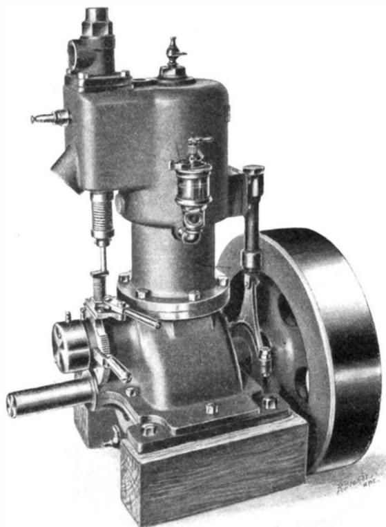
**A NOVEL, FOUR-CYCLE, REVERSIBLE, GASOLINE MOTOR.**
