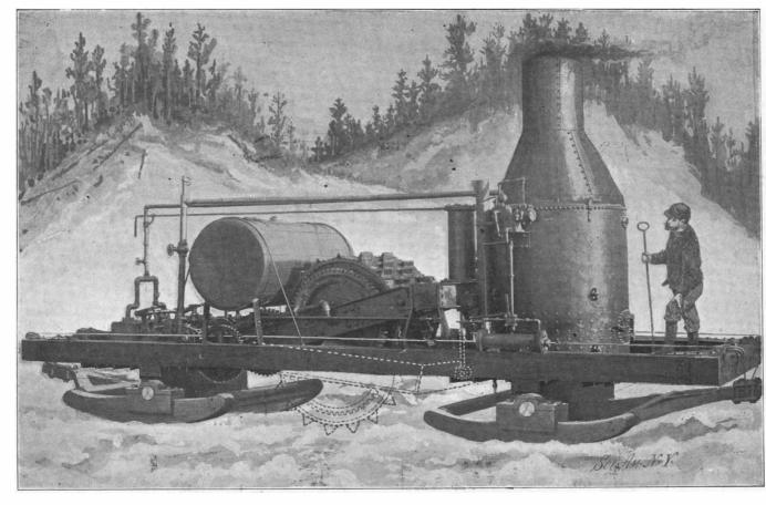
SNOW LOCOMOTIVE WITH HOUSING REMOVED TO SHOW THE OPERATIVE MECHANISM.
