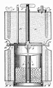
CROSS-SECTION OF ACETYLENE LAMP.
