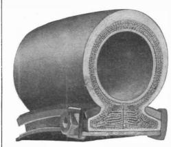
Inner Tube Cannot be Pinched Air Chamber All Above Rim Anyone Can Take Off and Put On
