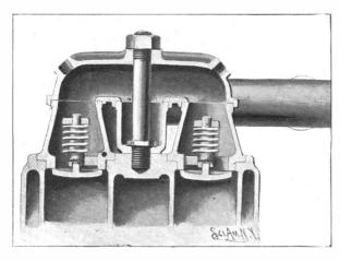
METHOD OF SECURING INLET VALVES.
