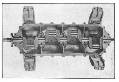
CRANK SHAFT AND CRANK CASE OF PEERLESS FOUR-CYLINDER MOTOR.
