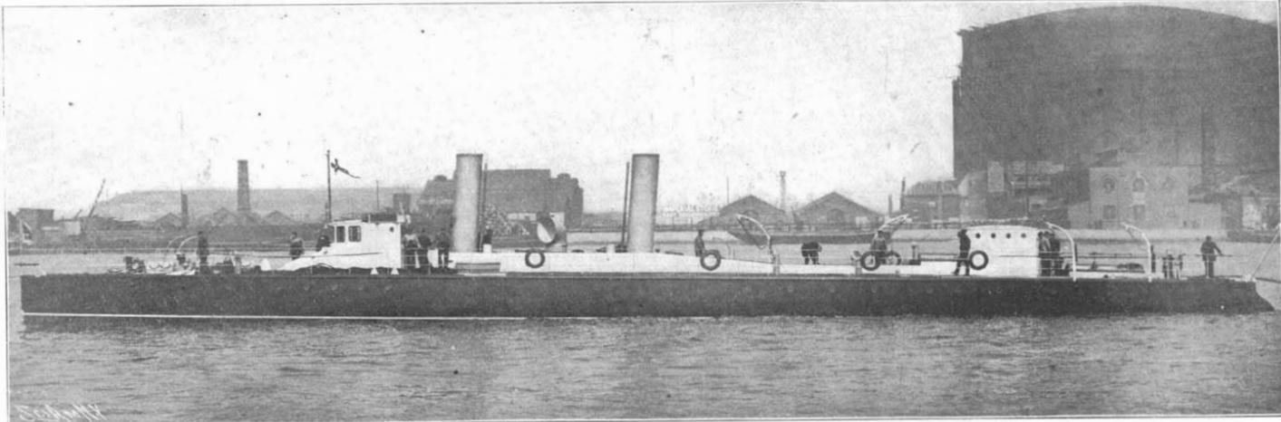
Length, 160 feet; beam, 16 feet; designed speed, 24 knots.
