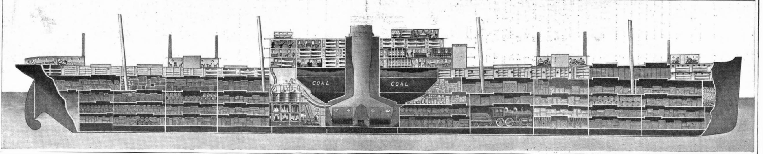
Length, 680 feet; breadth, 73 feet; depth, moulded, 56 feet; displacement on 83 feet draft, 33,000 tons; on 36½ feet draft, 37,000 tons.
