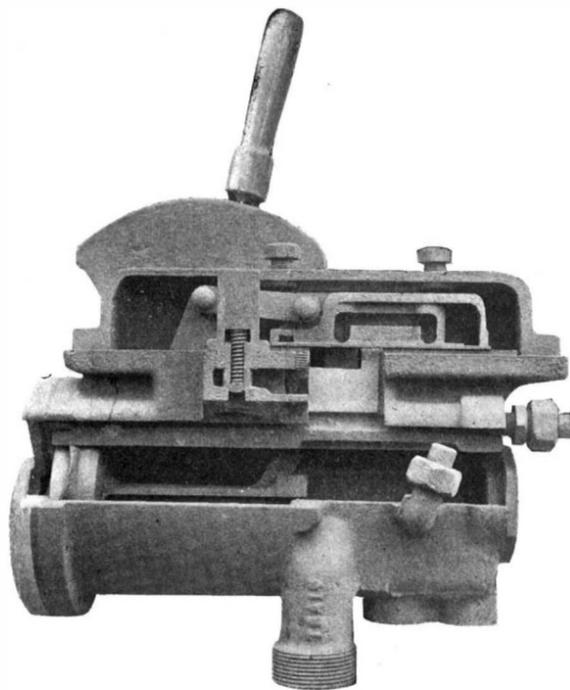
Fig. 2.—THE ENGINEER'S VALVE.
