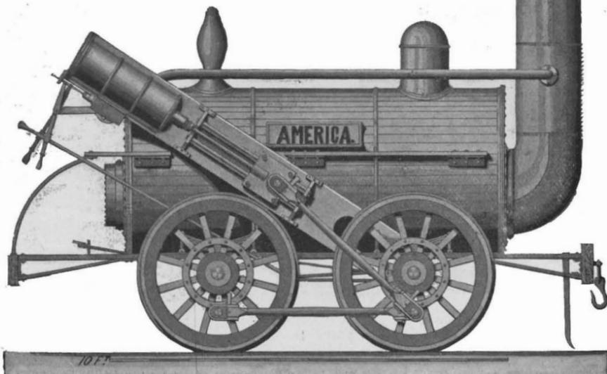
Fig. 3.—Stephenson's Engine. 1828. First Locomotive Seen in America
