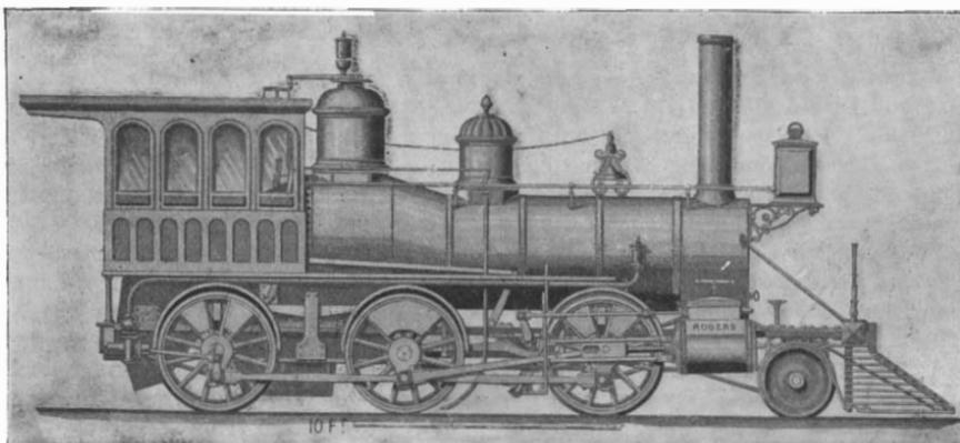
Fig. 8.—'Mogul' Engine. 1863. New Jersey R.R. & Transportation Co.
