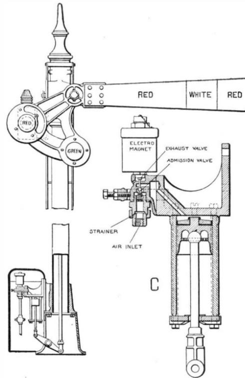
Fig. 3.—Details of Electro-Pneumatic Semaphore.
