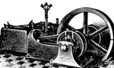
Double Cylinder, 50 h. p. and upward to 500.
