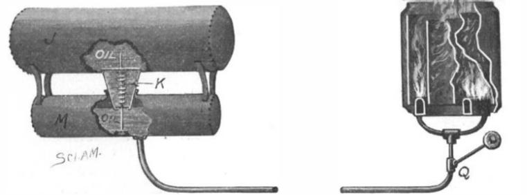
Detail of Automatic Oil Feed and Blue-Flame Burner.
