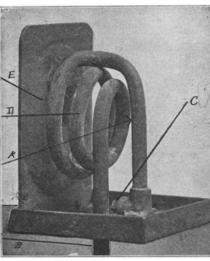
A—Orifice for flame. B—Oil inlet. C—Screw joint to pan. D Heating coil or retort. E—Flame deflecting plate.
