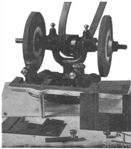
Fig. 1.—TOOL GRINDER WITH REST DETACHED.
