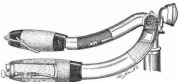
**HANDLE-BAR USED AS AN ACETYLENE GENERATOR.**
