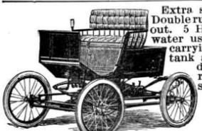
Extra strong road wagon. Double running gear throughout. 5 H. P. motor and no water used. Body free for carrying packages. Fuel tank and multiple oiling device sufficient to run 150 miles without stopping. Price \$850.
