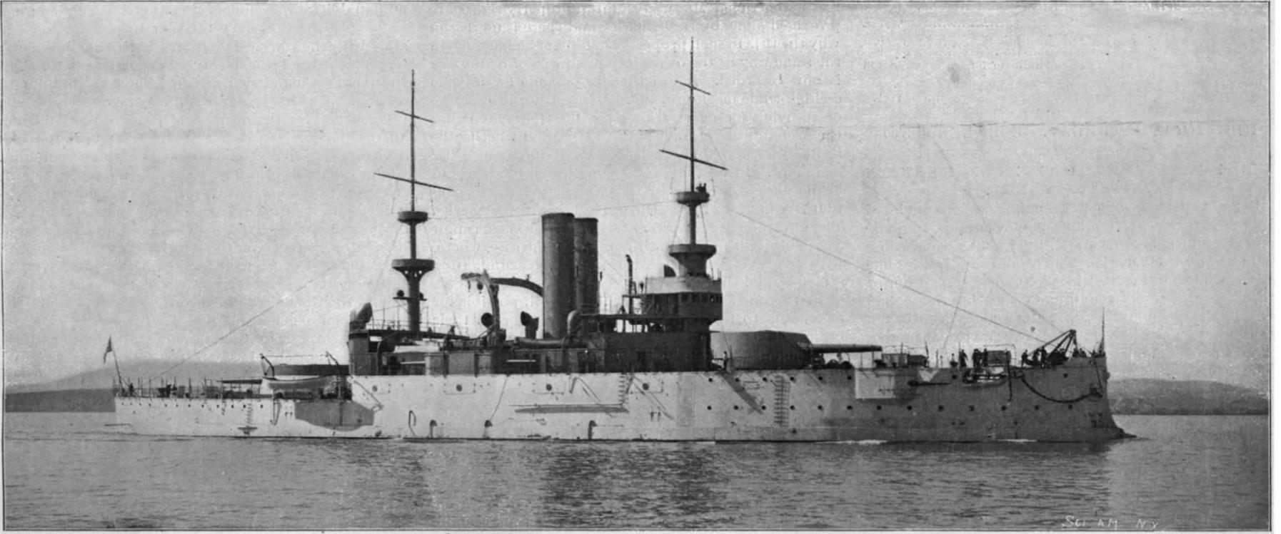
Displacement, 11,565 tons. Speed, 17.17 knots. Maximum Coal Supply, 1,440 tons. Armor: Belt, 16 to 4 inches; deck, 2 3/4 to 4 inches; gun positions, 15 inches. Armament: Four 18-inch; fourteen 6-inch rapid-fire; sixteen 6-pounders; four Colts; two 3-inch field guns. Torpedo Tubes, 4. Complement, 498.
