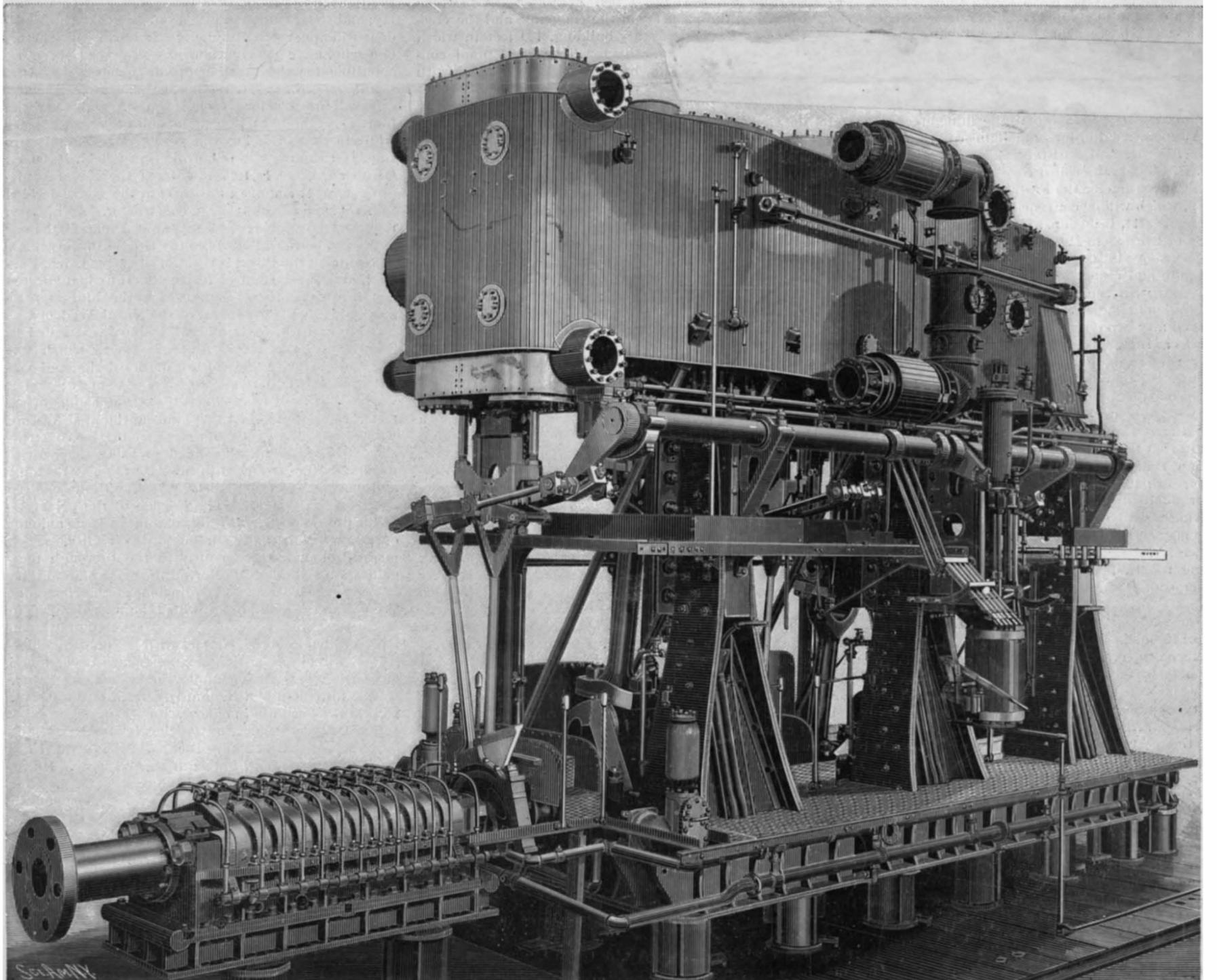
Cylinders, 33 1/2 inches, 51 inches, and 78 inches diameter by 48 inches stroke. Steam Pressure, 189 pounds. Air Pressure in firerooms, 1 inch. Indicated Horse Power, 12,321.
