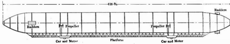
Fig. 2.—SIDE ELEVATION OF THE AIRSHIP.
