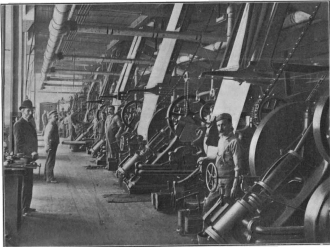
Cotton-Mill Printing-Machines Driven by Compressed Air Engines.
