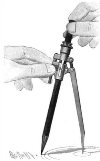
A SIMPLE COMPASS WITH A CALIPER SCALE.
