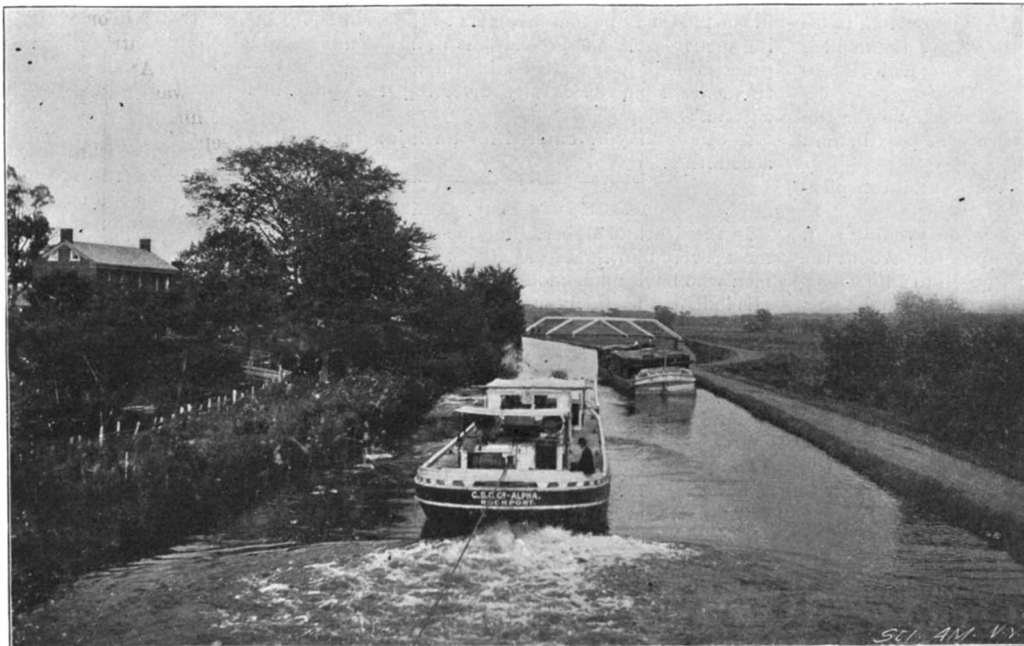
SELF-PROPELLING STEEL CANAL BOAT.
