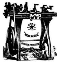
Star Lathes Foot power Automatic Cross feed 9 and 11-inch Swing. New and Original Features. Send for Catalogue B. Seneca Falls Mfg. Company, 695 Water St., Seneca Falls, N. Y.
