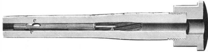
5.—Rifling Cutter Head in Barrel.
