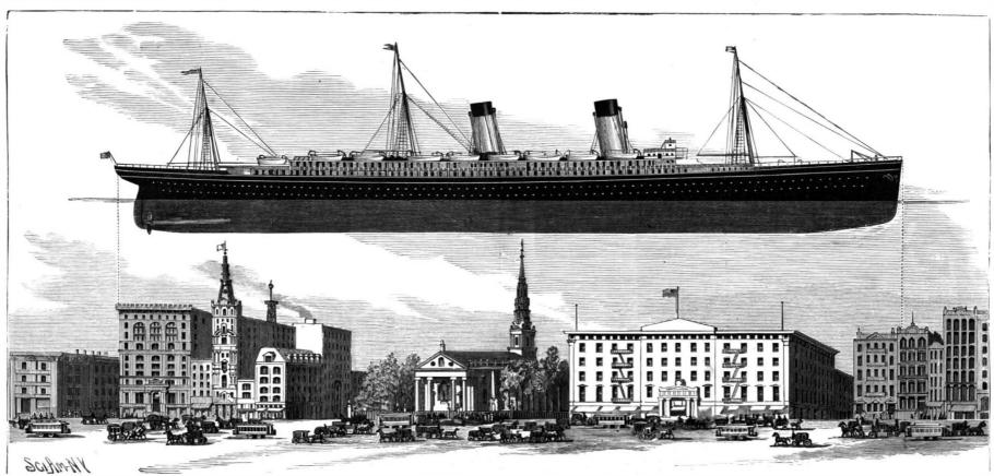
THE "OCEANIC" COMPARED WITH THE BROADWAY BUILDINGS AT CITY HALL PARK. Length, 704 feet; beam, 68 feet; depth, 49 feet moulded; 75 feet from keel to captain's bridge; displacement on 321/2 feet draught, 28,500 tons,
