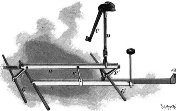
**Fig. 1.—SYSTEM OF COMPOUND LEVERS IN TYPE-BAR MECHANISM.**
