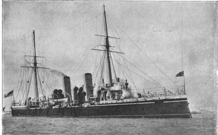
7.—Second-class Cruiser "Apollo." "Apollo" Class of Twenty-one Ships. Displacement, 3,400 tons. Speed, 20 knots. Normal Coal Supply, 400 tons. Armor: Deck, 1 inch on flats, 2 inches on slopes; gun positions, 4½ inches. Armament, two 6-inch and six 4.7-inch rapid-fire guns, eight 6-pounders, one 3-pounder, four machine guns, one boat gun. Torpedo Tubes, 4. Complement, 273. Date, 1892.
