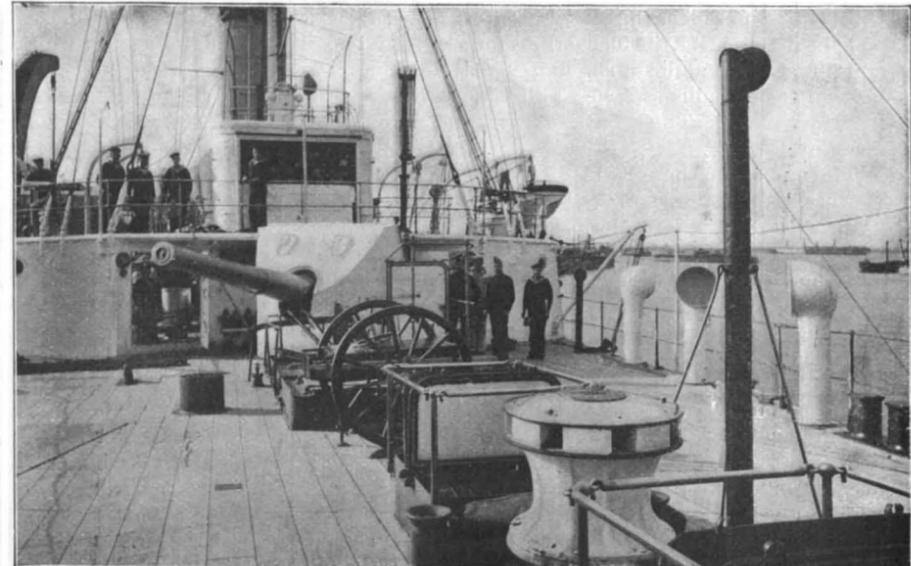
9.—Torpedo Gunboat "Speedy." "Speedy" Class of Eleven Vessels. Also four "Halcyon" type, 1,070 tons and 19 knots, and thirteen of "Gleaner" type, 785 tons and 20 knots. Displacement, 810 tons. Speed, 20.2 knots. Normal Coal Supply, 100 tons. Armor: Gun positions, 4½ inches. Armament, two 4.7-inch rapid-fire guns, four 3-pounders. Torpedo Tubes, 3. Complement, 91. Date, 1893.
