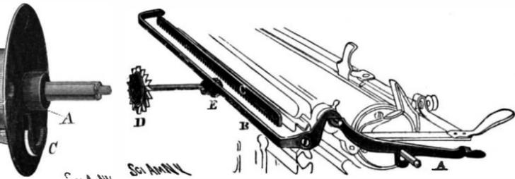
**Fig. 4.—ESCAPEMENT MECHANISM OF CARRIAGE MOVEMENT.**
