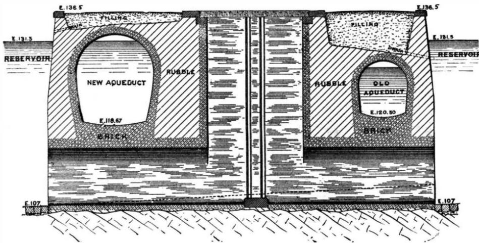
Fig. 2.—SECTION THROUGH DOUBLE CONDUIT ABOVE MAIN GATE HOUSE.
