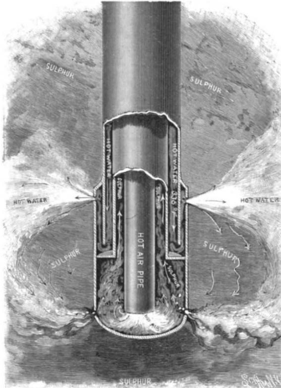
SECTION THROUGH INLET PIPE OF SULPHUR WELL.
