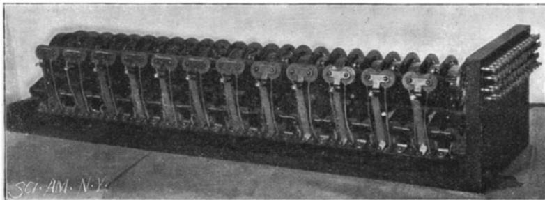
Fig. 3.—THE HOUTS TELEPHONE—SECTION OF CENTRAL OFFICE SWITCH.
