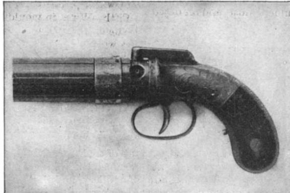
Fig. 4.—ALLEN "PEPPERBOX" (CAP SHIELD DISPLACED).
