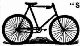
**"SWELL NEWPORT"** High-Grade Bicycles. Large Mannesman tubing, tool steel barrel hubs, barrel crank hanger. All turned parts finest quality tool steel. Strongest crown head in the world. Every machine fitted with S. & F. patent adjustable handle-bar. Any position obtainable without dismounting or the use of a wrench. **SNYDER & FISHER BICYCLE WORKS, Little Falls, N. Y.**
