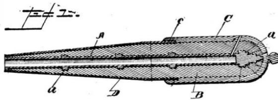
taper of the forward portion of the gun is forced over the rawhide until its inner end fits snugly within the groove or rabbet, c, of the cap, where they are secured together. The cap, C, is provided with the usual trunnions.
