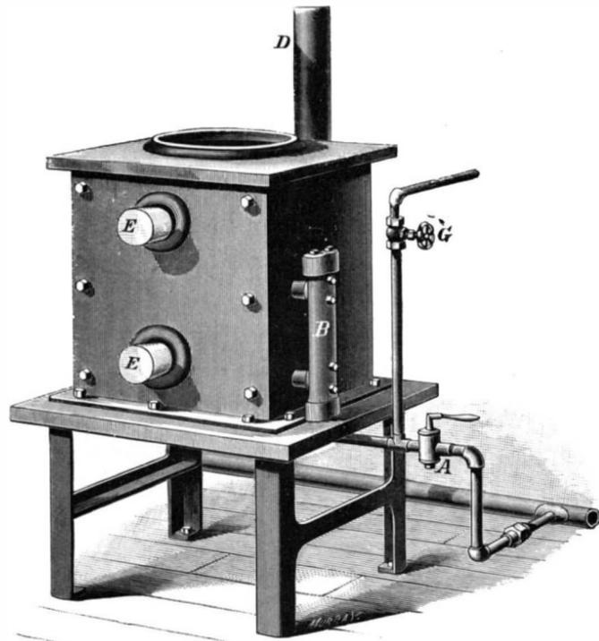
Fig. 11.—SOFT METAL FURNACE FOR LEAD HARDENING.
