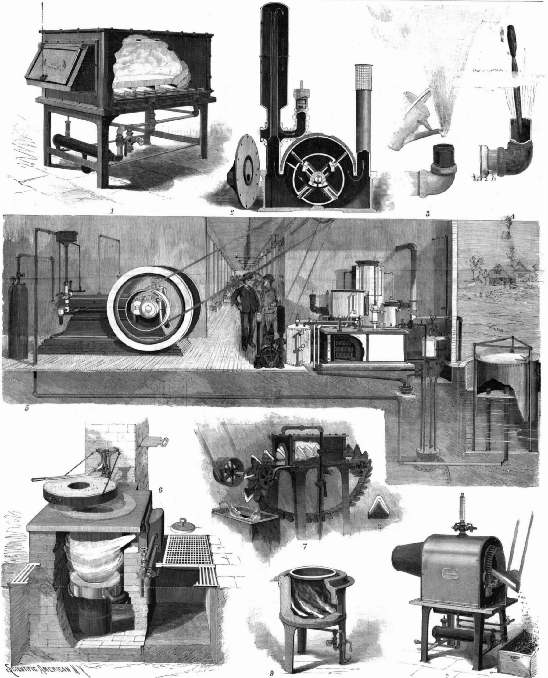
1. Large oven furnace. 2. Rotary blower. 3 and 4. Experiments with the blast. 5. The gas-producing plant. 6. Large melting furnace. 7. Furnace for tempering mowing machine cutters. 8. Soft metal furnace. 9. Furnace for bluing screws.
