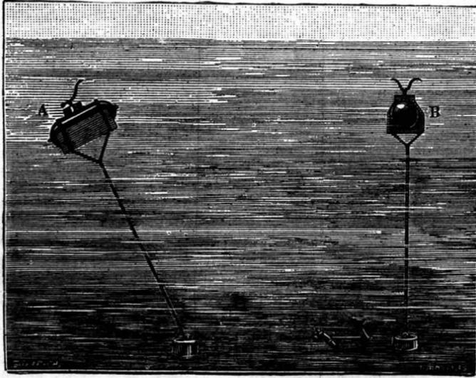
Fig. 1.—TORPEDO AT ANCHOR AND PLACED IN SUCH A WAY AS TO BLOW UP A SHIP COMING INTO CONTACT WITH IT.
