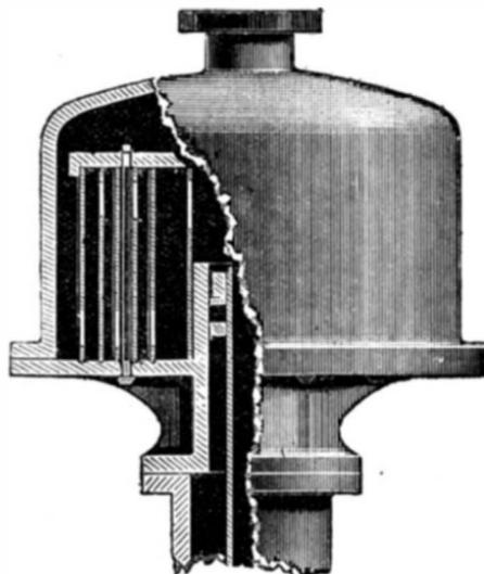
Fig. 5.—HALF ELEVATION AND SECTION OF THE SEPARATOR.
