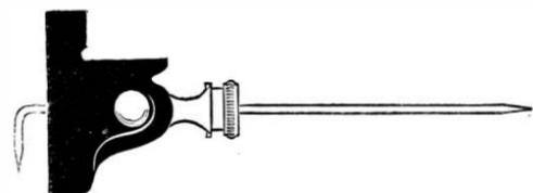
Fig. 5.—AS A SCRATCH GAUGE.
