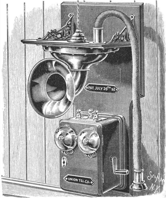
Fig. 2.—THE SIMPSON ACOUSTIC TELEPHONE—HORIZONTAL ARRANGEMENT.
