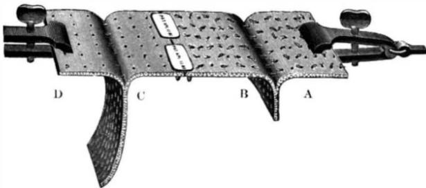
**TESTING STRENGTH OF RUBBER BELTS.**
